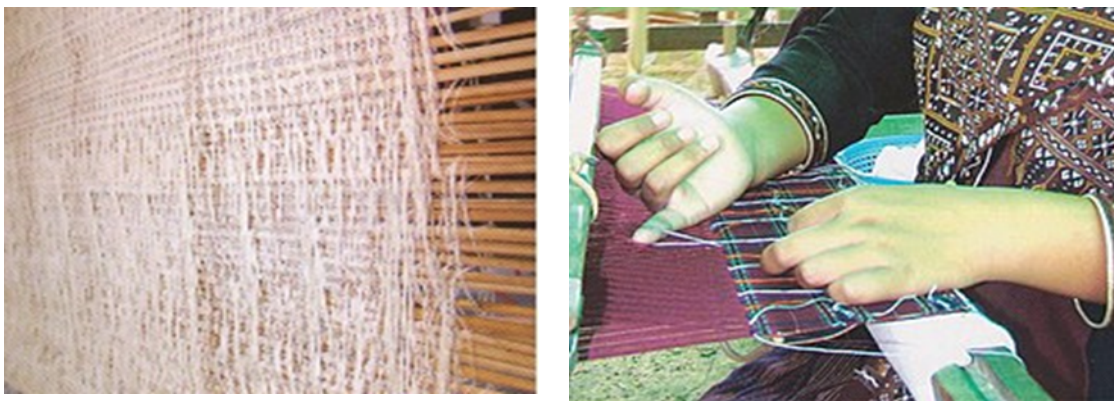
Figure 6. Method for collecting Khit patterns and the method of using the pinky finger to raise the warp yarn
