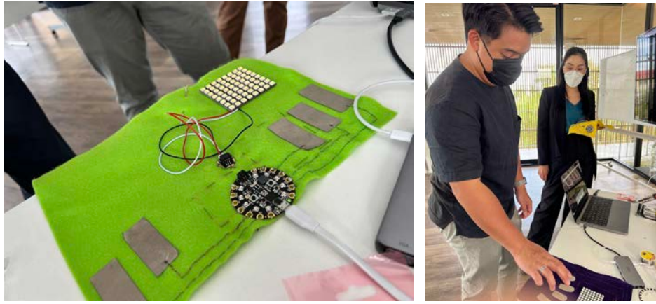
Prototype with five notes input & LED
